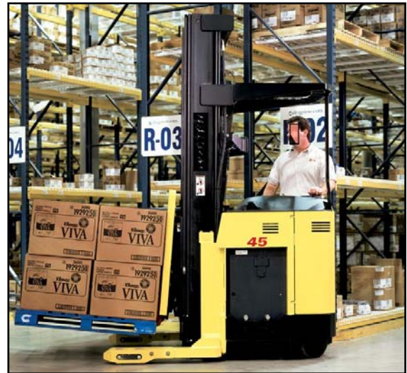
A narrow-aisle stand-up lift truck was backing down a warehouse aisle with a loaded pallet when the warehouse clerk in this incident walked into the aisle (stock photo of similar equipment).
