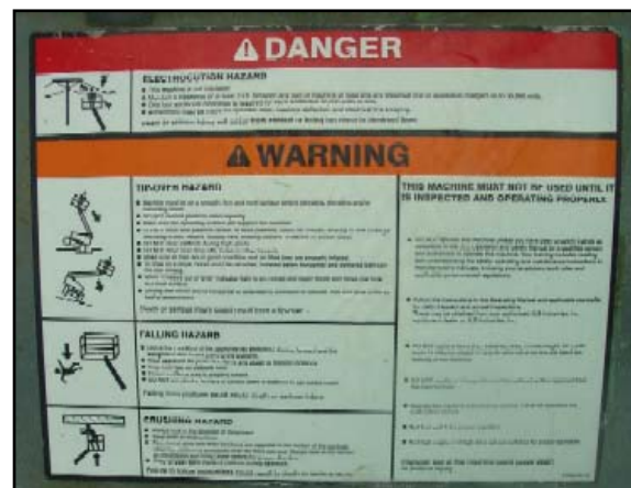
The warning label on the aerial platform illustrates the hazards of electrocution, falling, or striking an overhead obstacle.
