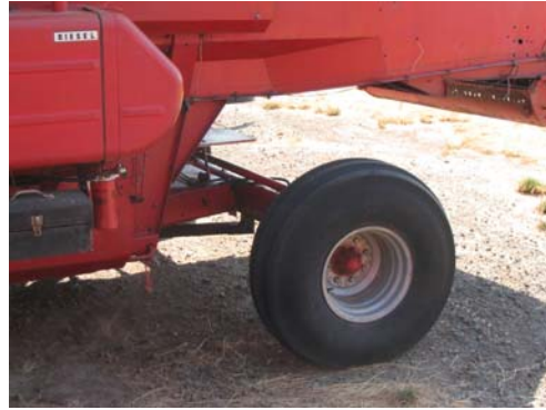
Photo 2. Space between rear tires and combine body and short narrow deflection shield.
