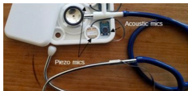
Early prototype of the "Telluscope" digital stethoscope developed by Dr. Schulman and his team.
