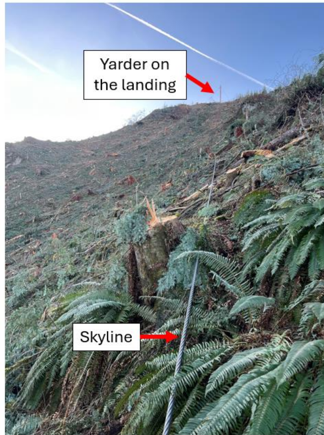
Image 3: Photo of the sloped terrain, skyline on the ground, and yarder on the landing above. (Photo courtesy of Oregon OSHA).
