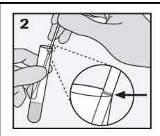
2. **ALIGN:** Remove the cap from the **cobas**® PCR Media Tube and lower the swab specimen into the tube until the visible scoreline on the swab is aligned with the tube rim. The bud of the swab should not be submerged into the liquid prior to breaking the shaft.
