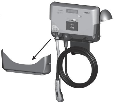
Insert the connector into the holster.
