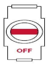
The gas is **off** when the lever is straight from left to right.
