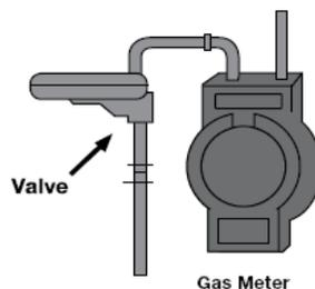
2. After you find the valve, turn it slightly. You'll know the gas is off when the lever is in a straight line from left to right on the pipe.
