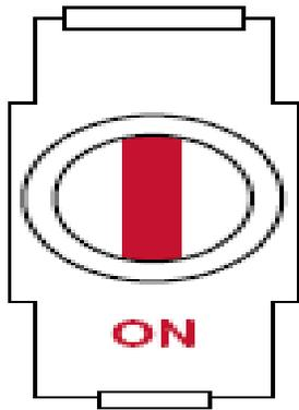
The gas is **on** if the lever is straight from top to bottom.
