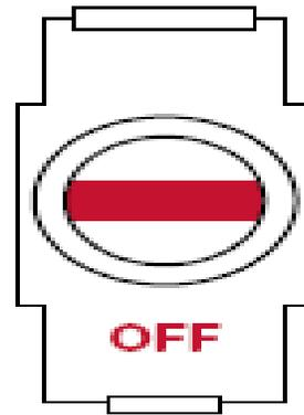
The gas is **off** when the lever is straight from left to right.
