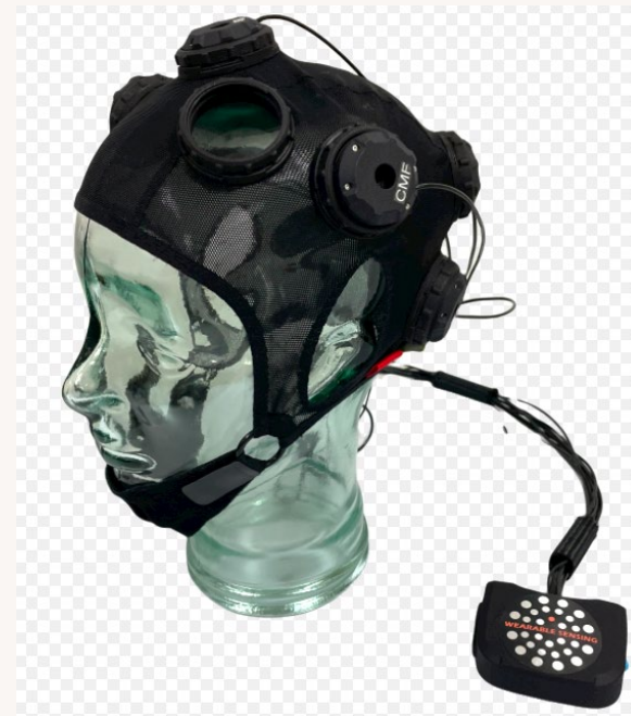
Flexible DSI dry electrode cap
