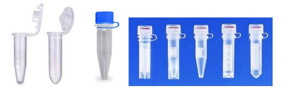
**NOT ACCEPTABLE:** cryovials are too wide to fit in our instrument and we will have to transfer the volume into an acceptable tube. Avoid collecting into these tubes (but do NOT thaw and transfer if already collected and frozen).
