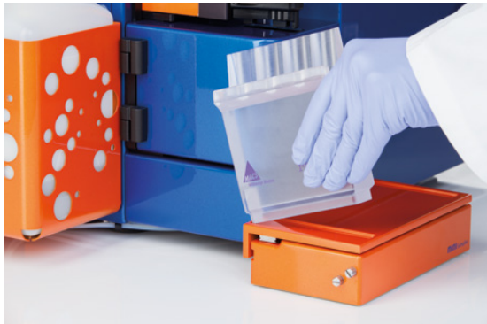
Figure 2.10: Secure the MACS Reagent Rack 4.
