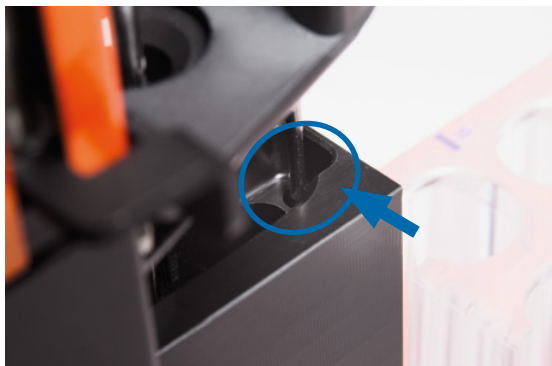
Figure 5.5: NEG needle in the washing station.
