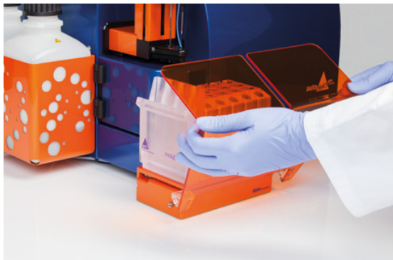
Figure 2.12: Attach the protective cover of the MACS MiniSampler Plus.
