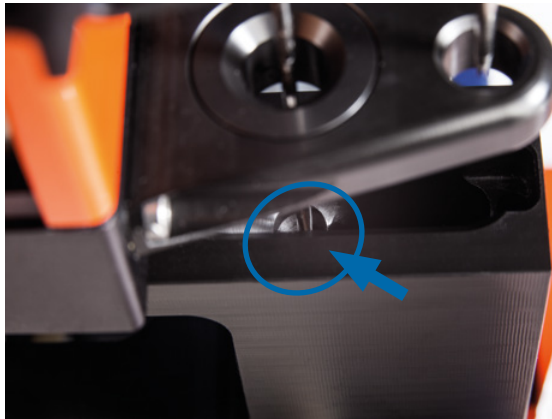
Figure 5.3: Uptake needle position in the washing station (arrow).
