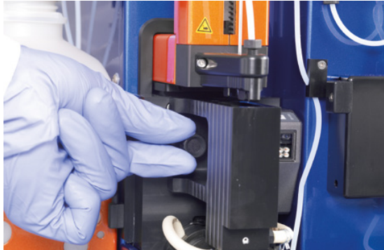
Figure 7.20: Dismantle the washing station.
