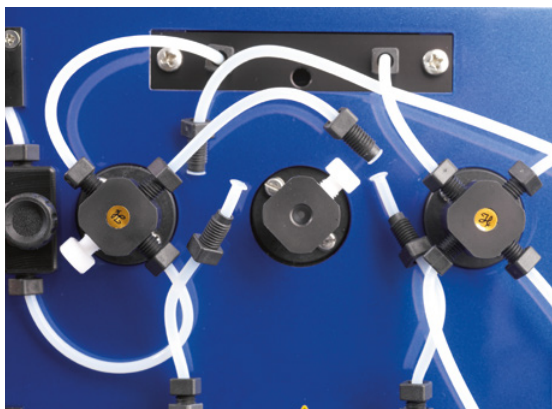
Figure 7.11: Unscrew the valve cover-screw and detach tubing and valve port locks or blind screws.
