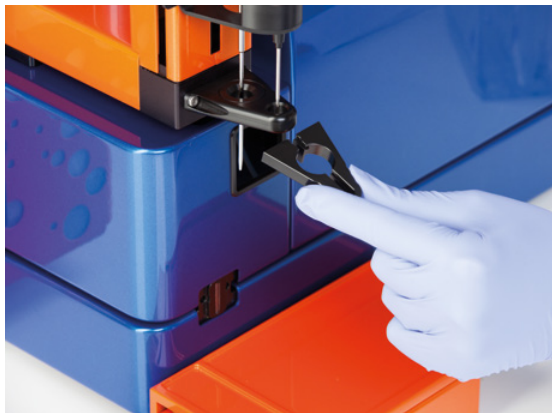
Figure 7.1: Removing the needle guard for cleaning.
