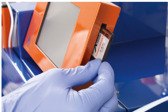
Figure 2.7: Insert the software memory card.
