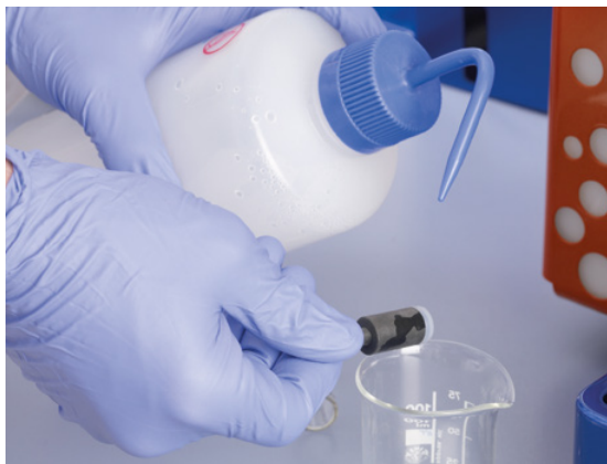
Figure 7.5: Wash the syringe with distilled water.
