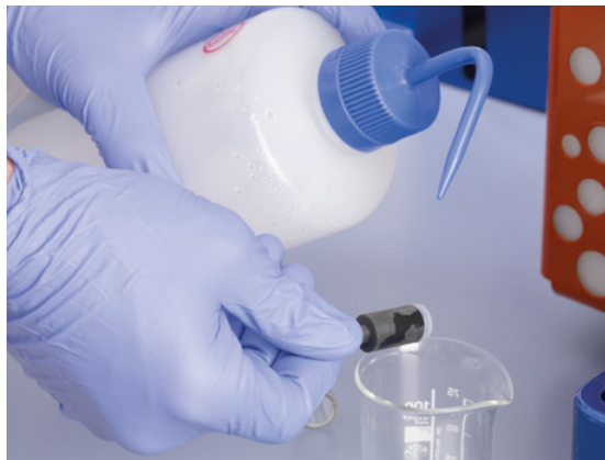
Figure 3.2: Humidify the plunger.
