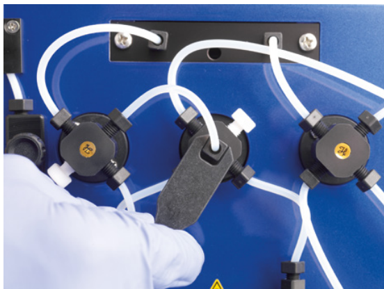
Figure 7.10: Unscrew the valve cover-screw.
