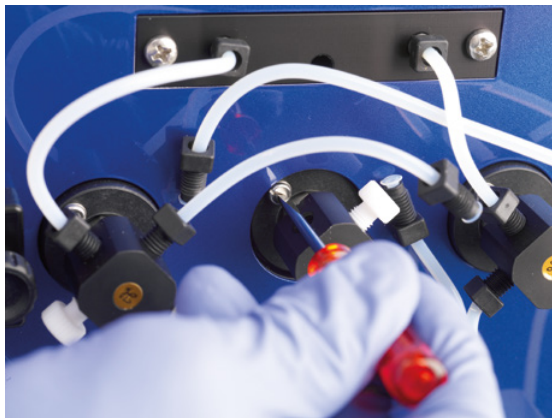
Figure 7.12: Loosen the valve screws.
