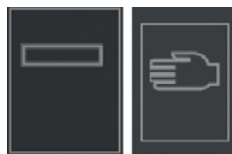
Figure 4.7: MACS MiniSampler Plus status graphic. Left: The MACS MiniSampler Plus was successfully installed. Right: No MACS MiniSampler Plus was detected.
