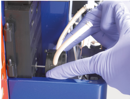
Figure 7.25: Detachment of the pump head.
