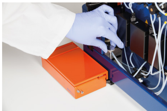
Figure 2.9: Secure the MACS MiniSampler Plus.
