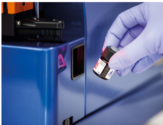
Figure 4.9: Scanning a reagent using the 2D code reader.
