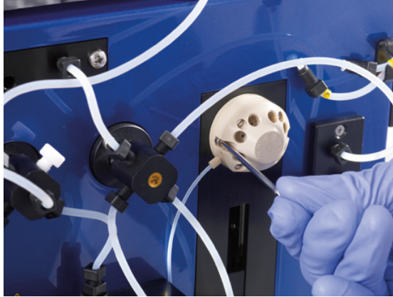
Figure 7.17: Unscrewing the dilutor valve's socket screws.
