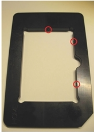
Terasaki plate adapter showing location of set screws
