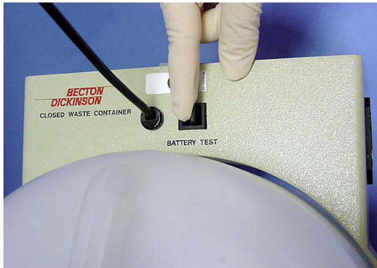
Figure 4-1 Battery Test switch
