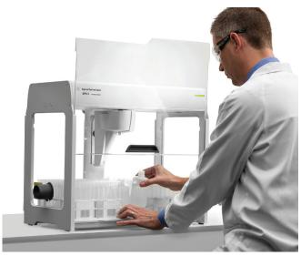
SPS 4 autosampler shown with optional integrated environmental enclosure. Front cover shown in fixed open position for easy access to samples.
