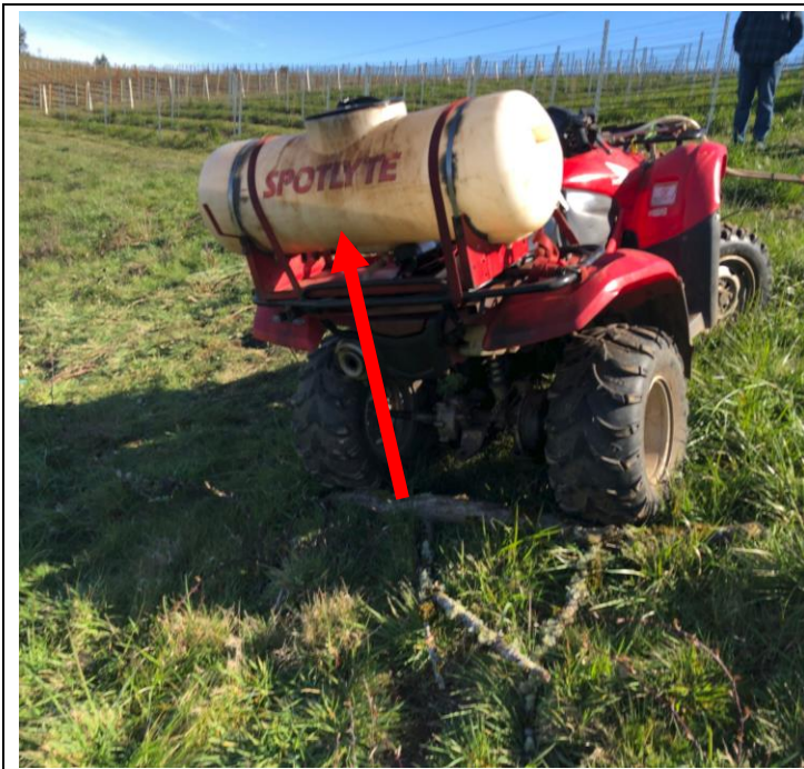
Image 2. Spotlyte™ tank attached to cargo area of ATV involved in incident. Note the liquid level in the tank indicates the slope of the terrain (red arrow).
