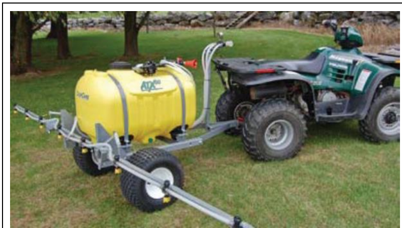
Image 4. spraying system mounted on a trailer, hitched to an ATV. (Photo credit: OSHA, 2015).
