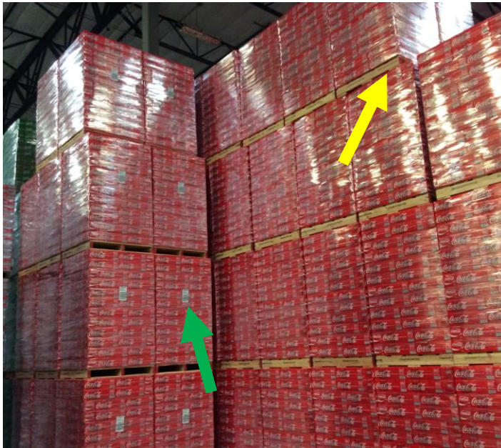
Image 2. Front of pallet row. Note top (4 th ) pallet layer offset behind 3 rd layer (yellow arrow). Also, note pallet labels with barcodes on shrink wrap, indicating this is the front of the pallet row (green arrow).
