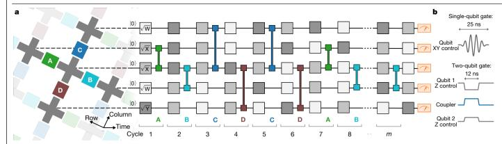
**Fig. 3** | **Control operations for the quantum supremacy circuits. a**, Example quantum circuit instance used in our experiment. Every cycle includes a layer each of single- and two-qubit gates. The single-qubit gates are chosen randomly from  $\{\sqrt{X}, \sqrt{Y}, \sqrt{W}\}$ , where  $W = (X + Y)/\sqrt{2}$  and gates do not repeat sequentially. The sequence of two-qubit gates is chosen according to a tiling pattern, coupling each qubit sequentially to its four nearest-neighbour qubits. The
