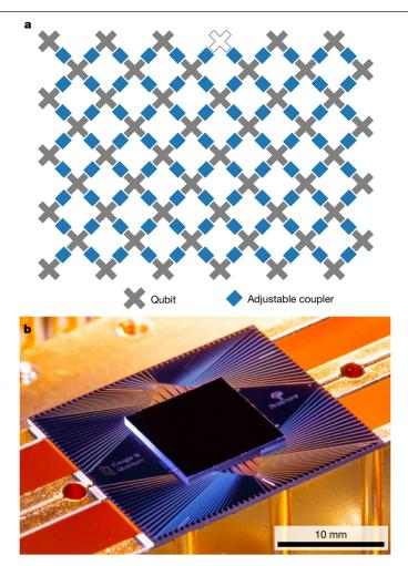
**Fig. 1** | **The Sycamore processor. a**, Layout of processor, showing a rectangular array of 54 qubits (grey), each connected to its four nearest neighbours with couplers (blue). The inoperable qubit is outlined. **b**, Photograph of the Sycamore chip.
