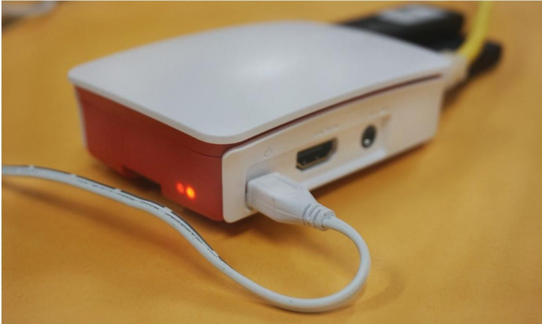
2. Once the Raspberry Pi powers on, connect your wireless device to the Raspberry Pi's **Wi-Fi** (pi-XXX). Find it under the Wi-Fi options list on your computer or tablet. Then, type in the password.
