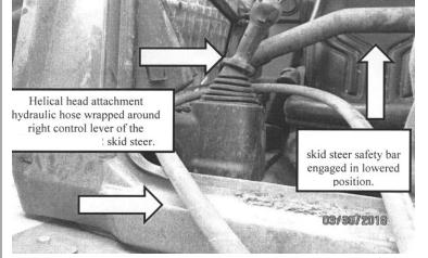
Photo 3: Hydraulic hose wrapped around control lever; (Photo courtesy of OR-OSHA
