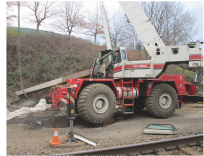
Figure 1: Crane cab struck by H-beam.
