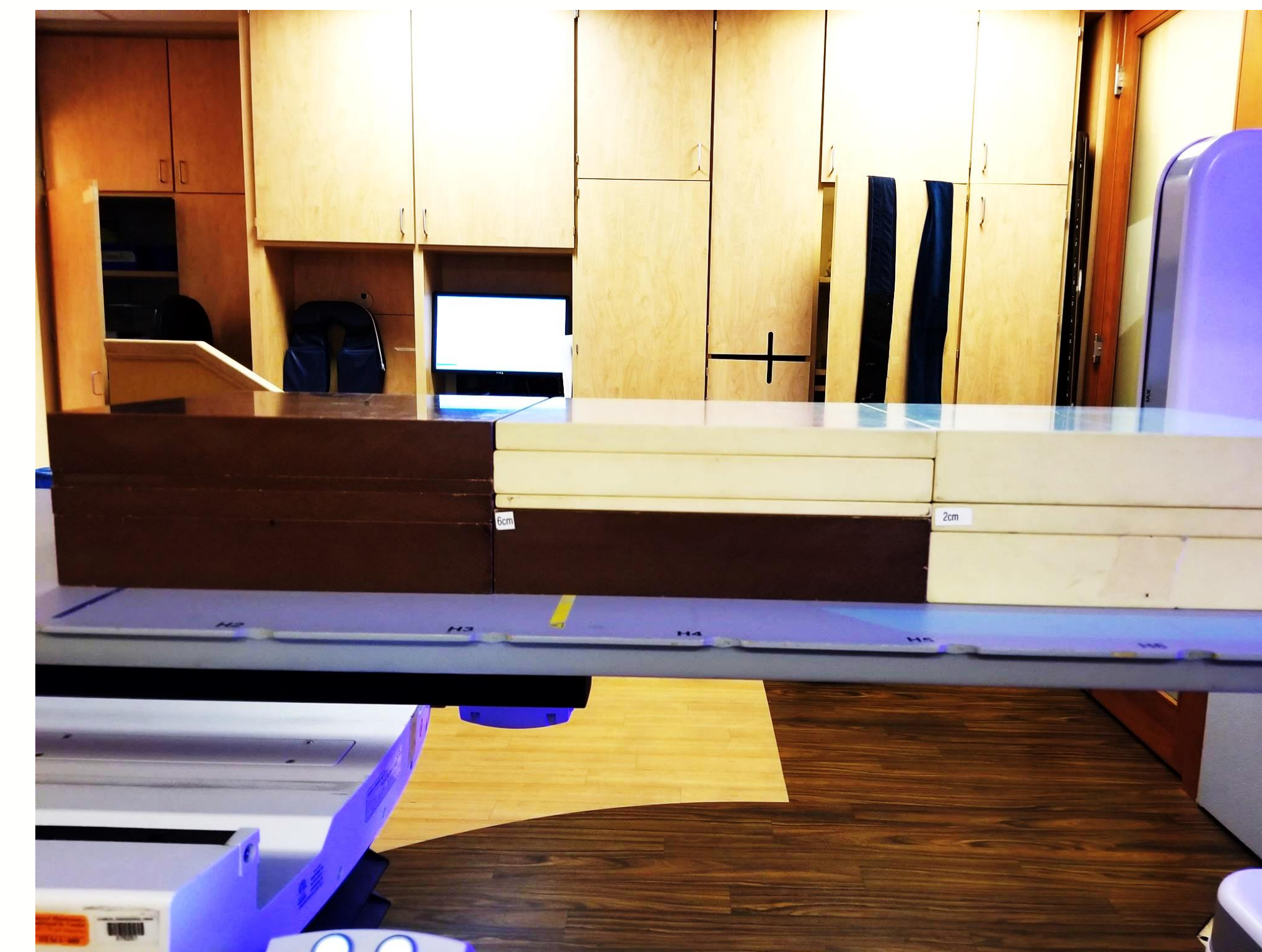
Figure 1b. Solid water phantom set up (6 MV, 10 x10 cm 2 , 100 cm SSD)
