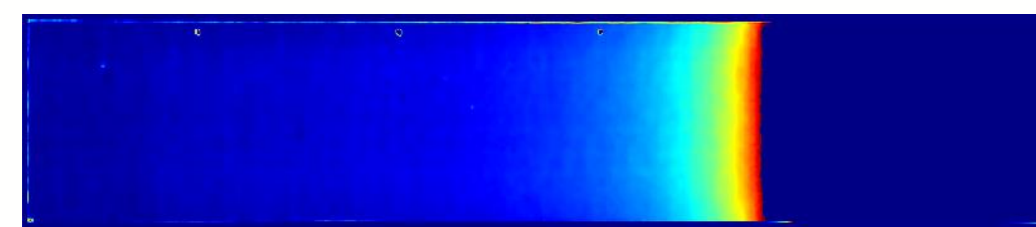
Figure 2a. Processed film #1 with calibration applied for distances of 5-15 cm away from the field edge
