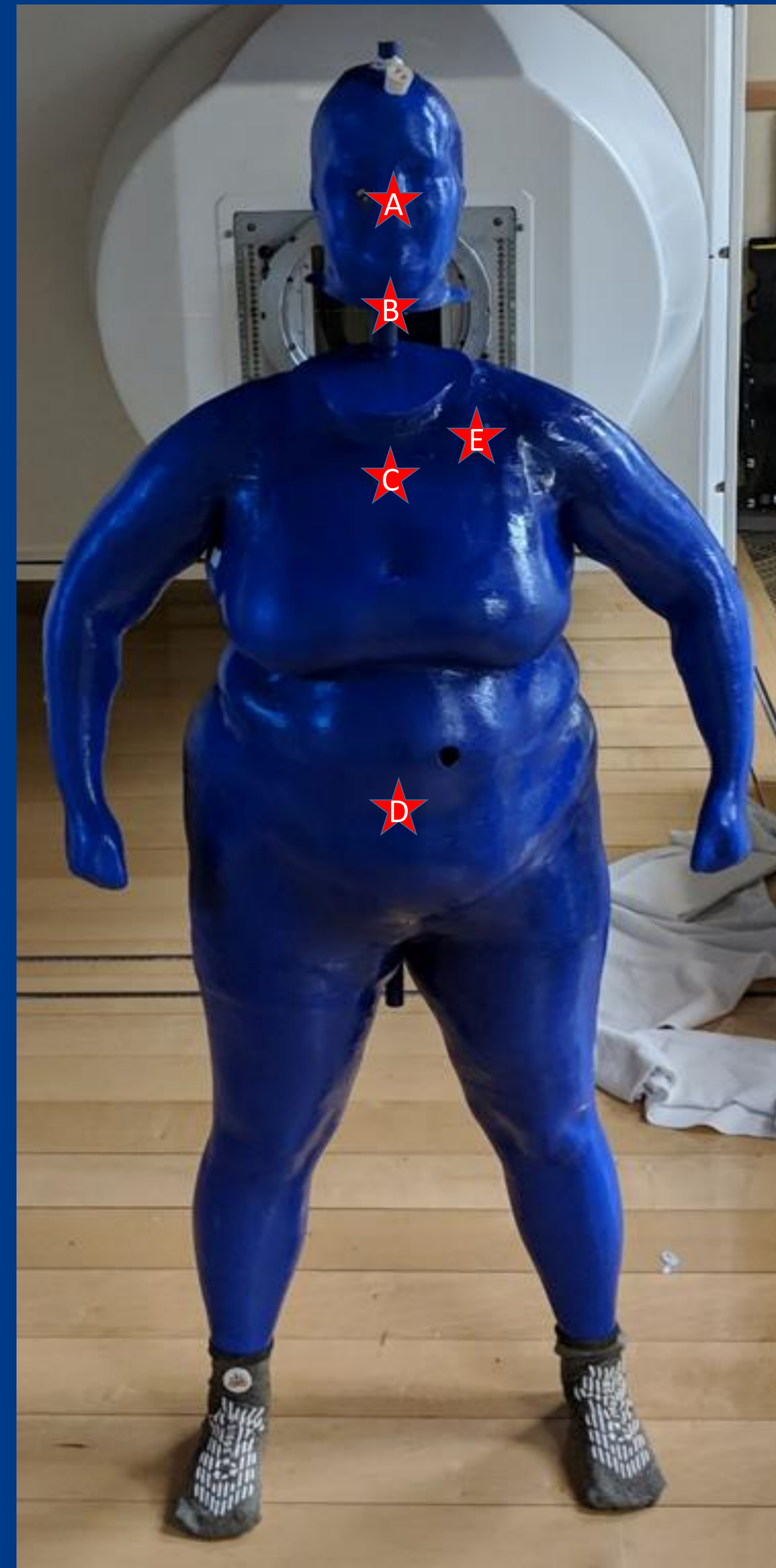
Figure 1. Photograph of 3D printed phantom shell. Labeled on the phantom are the approximate radiation detector placement locations for Isocenter (A), Thyroid (B), Esophagus (C), Fetus (D), and Pacemaker (E). Beams were delivered using left lateral fields of 2.8x2.8, 5.3x5.3, 7.8x7.8, 10.3x10.3, and 12.8x12.8 cm 2 for clinical photon (6 MV, 6 FFF), proton (170 MeV, 10cm SOBP), and neutron therapy. Detectors were placed inside the PVC pipe that lies along the central axis of the phantom for all measurements excluding the pacemaker. Buildup caps were employed for measurements taken at the pacemaker, giving an approximate depth of 5 mm.
