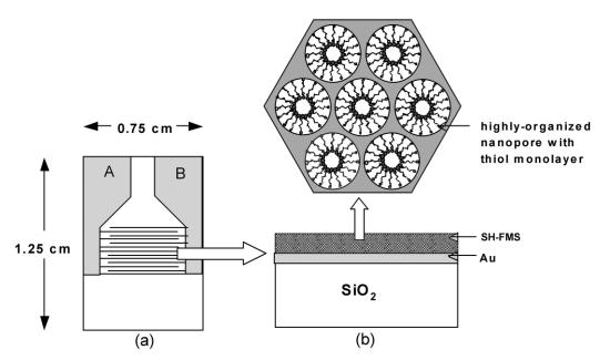
Fig. 1 A schematic of the gold electrode array with the SH-FMS thin film: (a) top-view of the array, and (b) side-view of the three-layer sensor (SiO<sub>2</sub>/Au/ SH-FMS).
