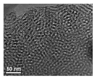
Fig. 2 TEM image of the mesoporous silica film.
