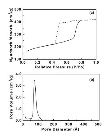
Fig. 3 BET analysis: (a) —  $N_2$  adsorption, ---  $N_2$  desorption, (b) the pore size distribution of the untreated mesoporous silica thin film.
