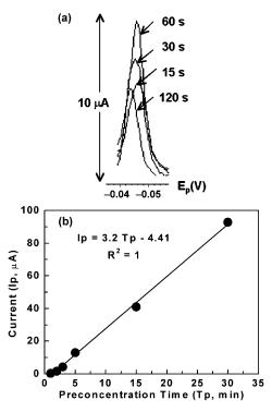
**Fig. 5** The effects of (a) electrolysis time and (b) preconcentration time on the voltammetric response for 1000 ppb Pb<sup>2+</sup> at the SH-FMS thin film modified gold electrode. Electrolysis/stripping media: 0.1 M HNO<sub>3</sub>.
