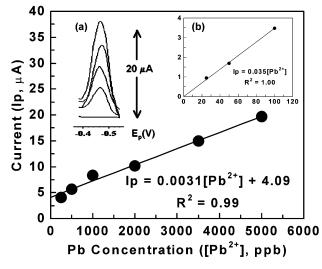
**Fig. 6** The calibration curve for Pb<sup>2+</sup>, measured after a 5 min preconcentration period with Inset (a) shows the representative voltammograms of Pb<sup>2+</sup> concentrations (in ascending order) of 0, 500, 2000, 3500, and 5000 ppb Pb<sup>2+</sup>, and Inset (b) shows the low-concentration-range calibration curve measured after a 30 min preconcentration period. All experiments were performed with a 60 s electrolysis period and 0.1 M HNO<sub>3</sub> as electrolysis/stripping media.
