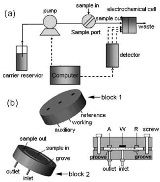
**Fig. 1a, b** Schematics of the metal analyzer (a) and the electrochemical cell (1.8 cm×2.4 cm in size; b); *solid lines* represent liquid lines and *dashed lines* represent electronic cable lines
