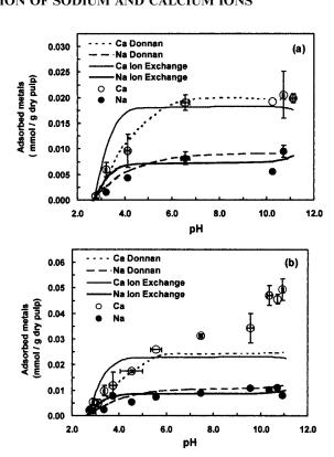
Competitive adsorption of Na+ and Ca+2 onto H-exchanged pulp at 25°C. (a) Bleached P3 pulp; (b) unbleached brownstock pulp. Process conditions are provided in Table 4. Solid lines represent multi-component ion exchange model predictions; dotted lines represent Donnan equilibrium model predictions. Error bars on adsorbed Na, adsorbed Ca, and pH are ±1.0 S.D. from triplicate measurements.
