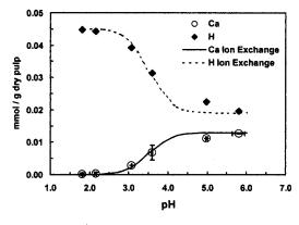
*Figure 4.* Adsorption of  $H^+$  onto Ca-exchanged bleached Perox pulp at  $25^{\circ}$ C. Process conditions are provided in Table 2. Solid lines represent ion exchange model predictions. Error bars on adsorbed Ca and pH are  $\pm 1.0$  S.D. from triplicate measurements.
