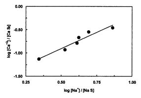
*Figure 7.* Distribution plot for Na<sup>+</sup> adsorption onto Ca-exchanged bleached P3 pulp at 25°C. Ion exchange parameter estimates are provided in Table 3.
