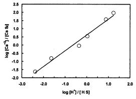
*Figure 5.* Distribution plot for H<sup>+</sup> adsorption onto Ca-exchanged bleached Perox pulp at 25°C. Ion exchange parameter estimates are provided in Table 3.
