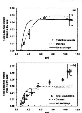
*Figure 10.* Total equivalents of Na<sup>+</sup> and Ca<sup>+2</sup> onto H-exchanged pulp at 25°C. (a) Bleached P3 pulp; (b) unbleached brownstock pulp. Error bars are  $\pm 1.0$  S.D. from triplicate measurements.
