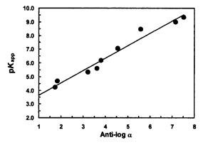
*Figure 3.* Plot of  $pK_{\rm app}$  vs. anti-log α for bleached P3 pulp at 25°C, using titration data presented in Fig. 2. From the intercept at anti-log α = 1, the intrinsic dissociation constant  $pK_{io} = 3.64 \pm 0.46$  (±1.0 S.D.); from slope,  $m = 0.902 \pm 0.062$  (±1.0 S.D.),  $r^2 = 0.97$ .
