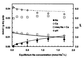
*Figure 6.* Adsorption of Na<sup>+</sup> onto Ca-exchanged bleached P3 pulp at  $25^{\circ}$ C. Process conditions are provided in Table 2. Solid lines represent ion exchange model predictions. Error bars on adsorbed Na are  $\pm 1.0$  S.D. from triplicate measurements; error bars on adsorbed Ca and pH were within the size of their respective data symbols.
