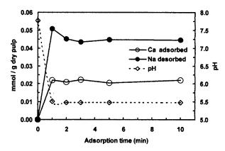
Figure 8. Adsorption kinetics of Ca<sup>+2</sup> onto Na-exchanged bleached P3 pulp at 25°C.
