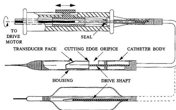
Fig. 10. Both US/atherectomy and US/balloon hybrids may require relative adjustment of transducer for full length views and 3D reconstruction. Modified Roberts handle (top) is equipped with a pressure seal to allow transducer positioning during atherectomy or angioplasty.
