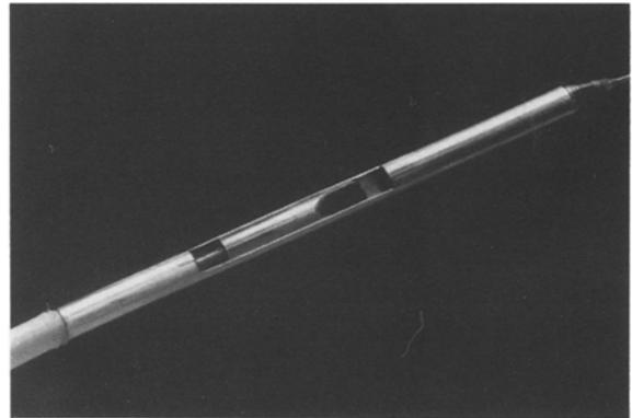
Fig. 3. Prototype US guided atherectomy catheter used for *in vitro* experiments. Transducer (dark ellipse) is seen at distal orifice. Cutting edge is on rear of transducer housing.
