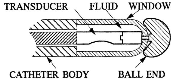
Fig. 5. Proposed US/recanalizer hybrid. Tissue is prevented from fouling transducer face by acoustic window. Ball end is driven by transducer at normal imaging speed of 600 RPM.
