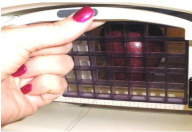
Carefully release compression and pull grid off wire
