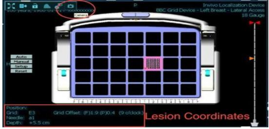
Coordinates of lesion – click on camera to take snapshot for printing The "Depth" will put the end of the needle exactly where you targeted NO MATH NECESSARY!
