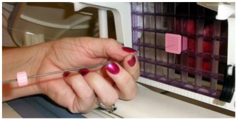
Pull the needle out over the wire leaving the wire in place
