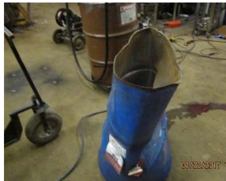
Photo 4. View of damaged drum following explosion; bottom of drum was blown off. (Photo courtesy of OR-OSHA)
