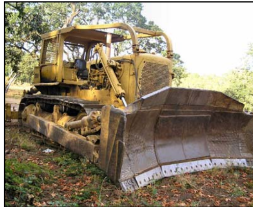
The Caterpillar D8H bulldozer in this incident unexpectedly rolled backward from a parked position.
