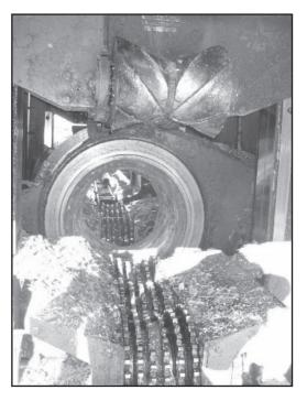
An incident with a debarker in 2008 involved maintenance on a debarker machine. The worker was crushed under the heavy press roll (at top) when hydraulic pressure was released.
