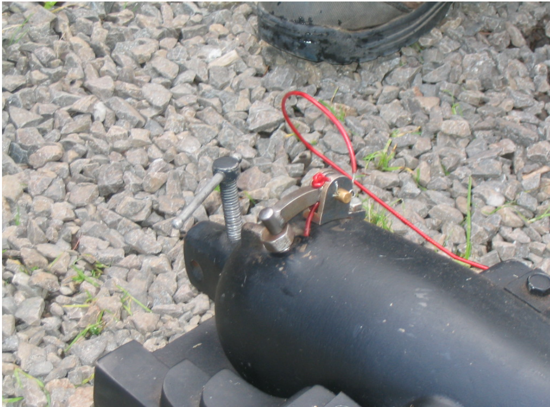
Photo 3. This photo shows a solid steel cannon in use at another of this employer's youth camps. This cannon is equipped with a 'slap hammer' for firing. Problems encountered with other firing methods, i.e., touchstick, fuse, loose powder, etc. are eliminated. The person firing the cannon typically stands 4-5 feet from the cannon and pulls a lanyard to set off a small cap-like primer charge in the cannon's touchhole.
