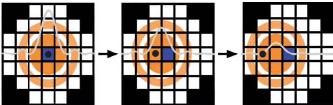
Fig. 3: The object (grey spot) is illuminated by a point source (blue) and will emit photons that will be recorded on an array detector. As the sample is scanned (in the direction of the arrow), not only will each detector element (squares) see the whole image, but they would probe the Airy disk (displayed in orange) as well. The obtained detection PSFs (grey curves) would be shifted and their amplitudes decrease with increasing shift.
