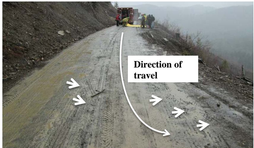
Figure 2. White bold arrows point to the tire tracks on the road leading off the edge. White line shows the trucks direction of travel.
