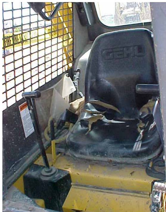
Photo 2. Position of safety bar following the incident.
