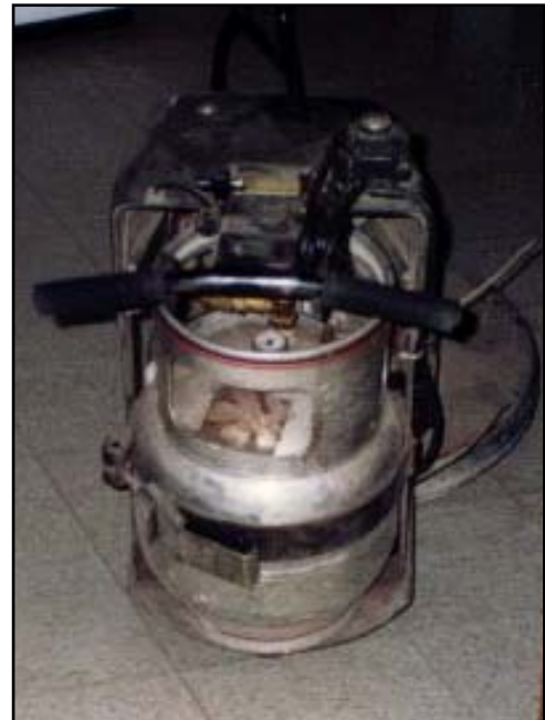
The propane-powered buffer used in this incident produced high levels of carbon monoxide.
