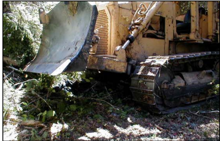
The final resting position of the bulldozer shows the front blade was raised about 1 ft off the ground when parked.
