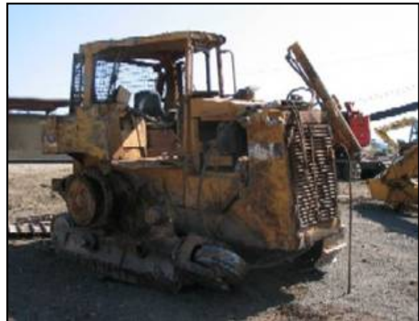
The D6H Caterpillar following the incident shows noticeable damage – missing the front blade, rear grapple, and tracks – but the operator's cage is relatively intact.
