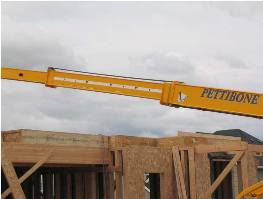
**Photo 4.** In upended position, the boom is extended between "D" and "E" load rating. Weight of load was calculated to be 3600-3800 lbs. extended ~24ft. The maximum load range at this reach and arc is 2000-3000 lbs.
