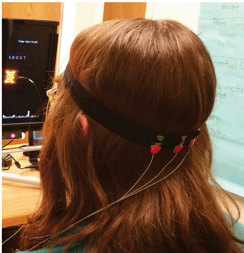
Figure 4. Shuffle Speller electrode placement.
