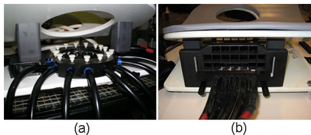
FIG. 6. (Color online) The patient interface is a circular array of fibers that couples into a standard MR breast coil (a) although parallel plate geometries are also under consideration (b).
