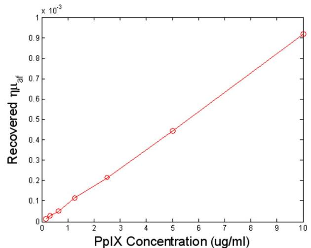
**Fig. 3** The reconstructed quantum yield multiplied by the fluorophore absorption coefficient is shown within the region of the phantom, for a range of increasing PpIX concentrations. The linearity of the recovery provides a reliable way to calibrate the concentration from within tomographic images.
