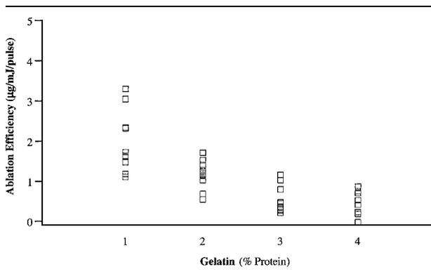
**Fig. 5.** Mean ablation efficiency of the gelatin clot models. The gelatin models varied significantly (ANOVA,  $p < 0.001$ ) in ablation efficiency, with significant differences between 5–10% and 15–20% protein concentrations.
