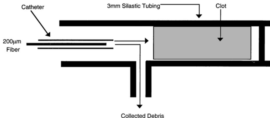
**Fig. 1.** The in vitro laser thrombolysis experimental set up. Laser energy is delivered through the fluid core catheter to the clot in the ablation chamber. The ablation chamber contains a 3 mm inner diameter section of tubing which holds the clot and has a bypass for the collection of effluent.
