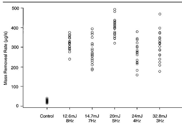
**Fig. 6.** Mass removal rate of reconstituted model A clot at varying laser pulse energy (mJ) and repetition rates (Hz). Average power was approximately 100 mW. There were statistically, but not clinically significant differences among the groups.
