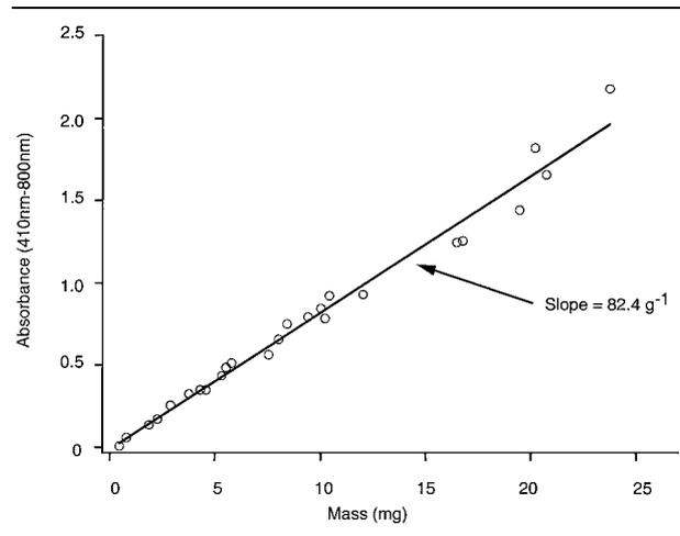
**Fig. 2.** Calibration curve. Absorbance difference between 410 nm and 800 nm vs., mass (g), slope ( $k$ ) =  $82.4 \text{ g}^{-1}$ . Each clot model formulation had its own calibration curve value. Absorbance values were measured at 510 nm and 800 nm for gelatin phantoms. The  $r^2$  value for all linear regressions was  $\geq 0.90$ .
