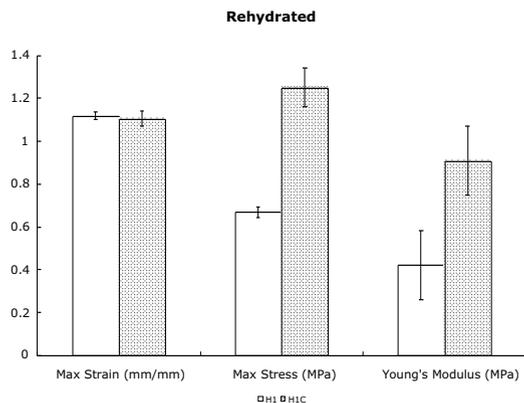
**Figure 8** Ultimate strain, stress and Young's modulus data of cured EH1C (grey bar) and non-cured EH1 elastin (white bar). Although the maximum strain remains unchanged, curing significantly increases the maximum stress and Young's modulus ( $p < 0.01$ ).
