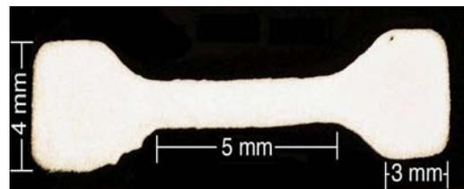
**Figure 3: Typical dumbbell shaped specimen**
