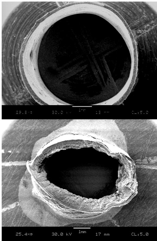
**Figure 6:** SEM top down view of cross section of distal portion of uncured elastin conduit EH1 (left). SEM top down view of cross section of distal portion of cured elastin conduit EH1C (right). Note the reduction in wall thickness caused by compaction of the elastic fibers indicated by the arrows. Bar 1 mm
