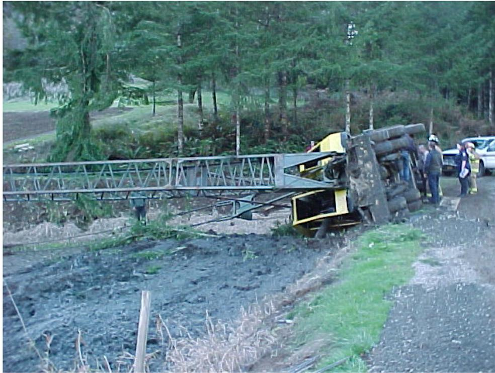
Photo 2. Crane topples over, crushing worker, while dredging dry fish pond.
