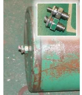
Gas pressure release valve in incident, believed to be damaged when accumulator flew off the table. Shown removed next to a new valve.
