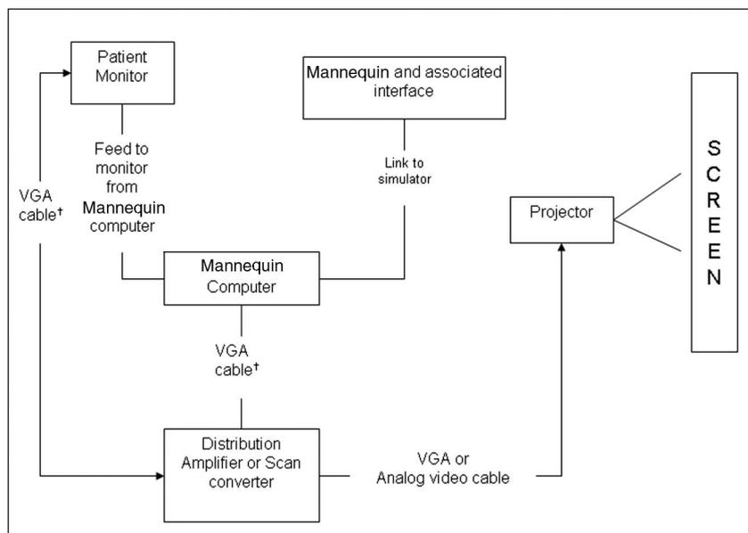
† VGA cable source and routing will vary depending on mannequin manufacturer. Several different layouts are represented here.
