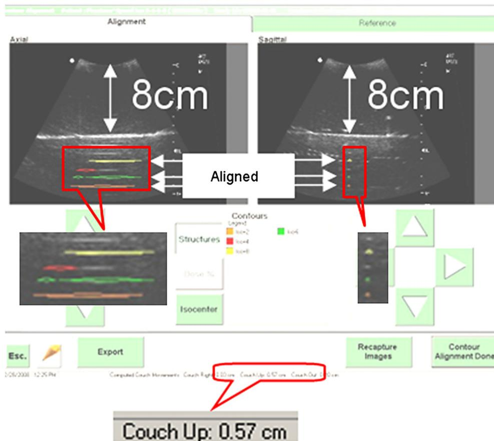
**Figure 4.** A screen snapshot of BAT, post-contour alignment, for the phantom with 8 cm fat material on top. Both axial and sagittal US images of the target-simulating wires were correctly aligned with the contours in the depth direction (A/P) after a 5.7 mm couch up shift.
