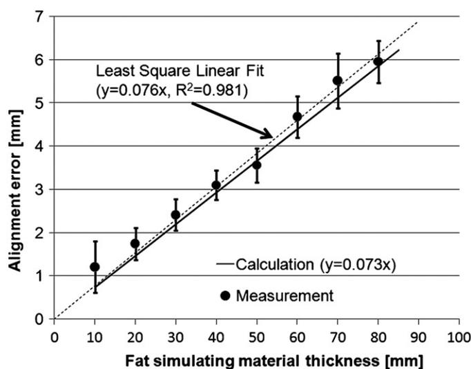
**Figure 5.** Comparison of measured alignment errors (caused by speed artifact) with the calculated values for eight different thicknesses of the fat-simulating material. The measurements and the calculations one agree within standard deviation or a maximum deviation of 0.47 mm.
