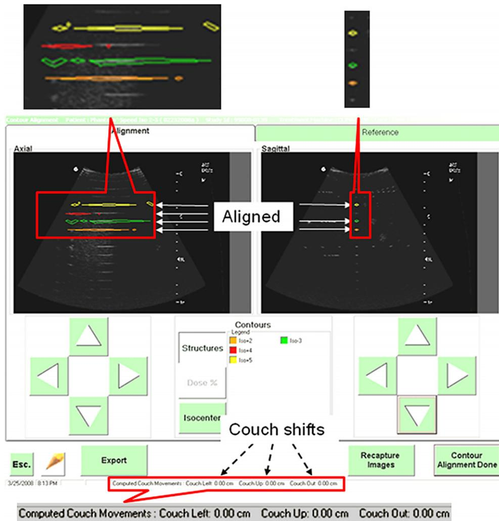
**Figure 2.** The alignment of the phantom target-simulating wires without any fat- or tissue-simulating material. The zero couch shifts indicated a perfect system calibration.
