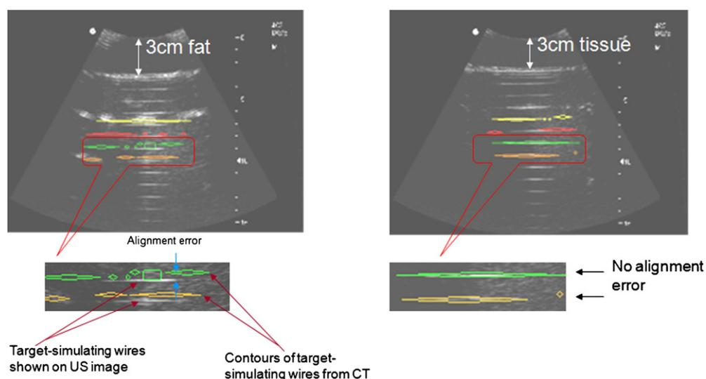
**Figure 3.** US axial images of the phantom with either 3 cm fat- (a) or tissue-simulating material (b) on top. No software manipulation of the contour alignment has been performed. (a) The US image of the target wires and the contours are not correctly aligned for the case of fat-simulating material and would require a 2.5 mm vertical shift to correct. (b) In contrast, the US image of the target wires and the contours are perfectly aligned for the case of tissue-simulating material.
