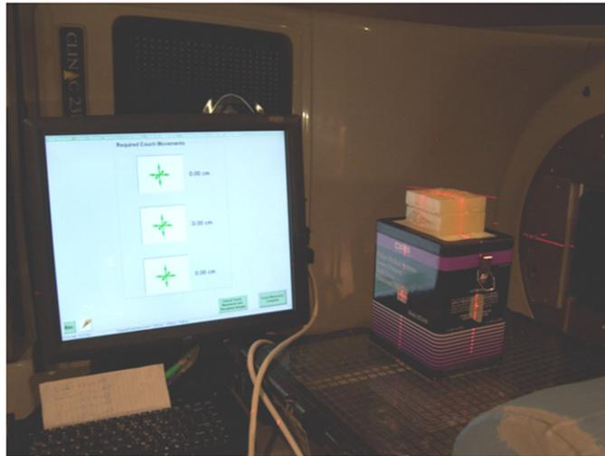
**Figure 1.** Experimental setup of the US phantom and BAT SXI system. Two layers (3 cm and 2 cm) of fat-simulating material are shown stacked on top of the US phantom.
