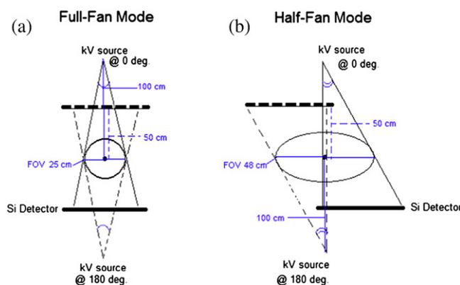
Fig. 2. Cone-beam CT imaging geometry: (a) full-fan mode, (b) half-fan mode.
