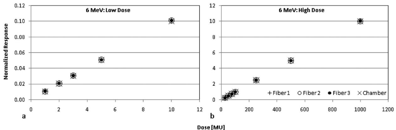
FIG. 2. Response curves of three FOCDs and a reference ionization chamber for (a) low doses (range: 1–10 cGy) and (b) high doses (range: 11–1000 cGy) for the 6 MeV beam, measured at standard calibration settings; the linearity coefficient  $R^2$  is 1.000 for the FOCDs.
