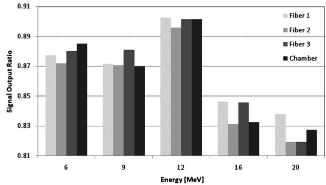
FIG. 5. Energy response of four detectors: Three FOCDs and a reference ionization chamber. Energy response was computed as the ratio of each detector’s signal output at two depths; a specified depth and at depth of maximum dose, for a  $10 \times 10 \text{ cm}^2$  cone size and 100 cm SSD.
