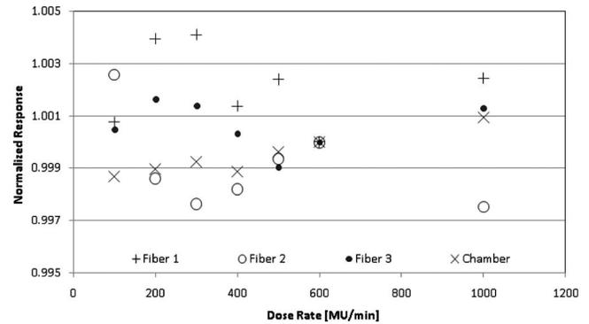
FIG. 3. Dose-rate response of three FOCDs and a reference ionization chamber under pulsed radiation from the 6 MeV electron beam. Dose-rate response was normalized to unity by the response at 600 MU/min.
