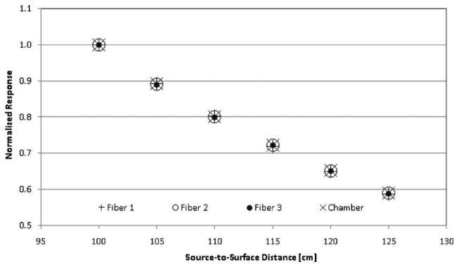
FIG. 4. Dose per pulse response of three FOCDs and a reference ionization chamber under pulsed radiation from the 6 MeV electron beam. Dose per pulse response was normalized to unity by the response at 100 cm source-to-surface distance.
